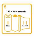
Final width of film as measured on the flat end of a round bale should, with 500mm film be 380mm-420mm, and with 750mm film be 580mm-620mm. Should film width vary outside these limits, stop wrapping and ascertain cause. Ensure prestretch unit rollers are regularly cleaned in accordance with wrapper manufacturer's instructions.
