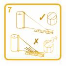
Ensure that the blade of the balewrapper's cutting mechanism is maintained in order to ensure a clean film cut after wrapping and thus avoid long film tails.
