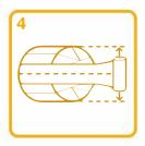
The height of the pre-stretch unit should be adjusted so that the centre points of the bale and film reel are horizontally aligned. Thread and attach film as per wrapper instructions.
